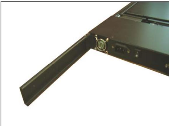
2. Fasten the extended brackets with the supporting brackets and the chassis.
