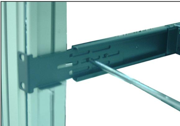
3. Screw the L brackets with the extended brackets. Adjust the length of L brackets according to your needs.
