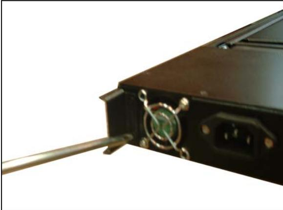
1. Fasten the supporting brackets with the chassis.
