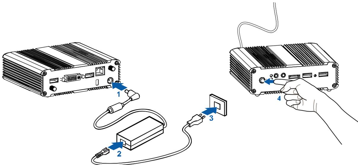
Figure 7 Turning on the system
