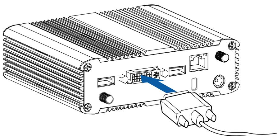
Figure 4 Connect the DVI cable
