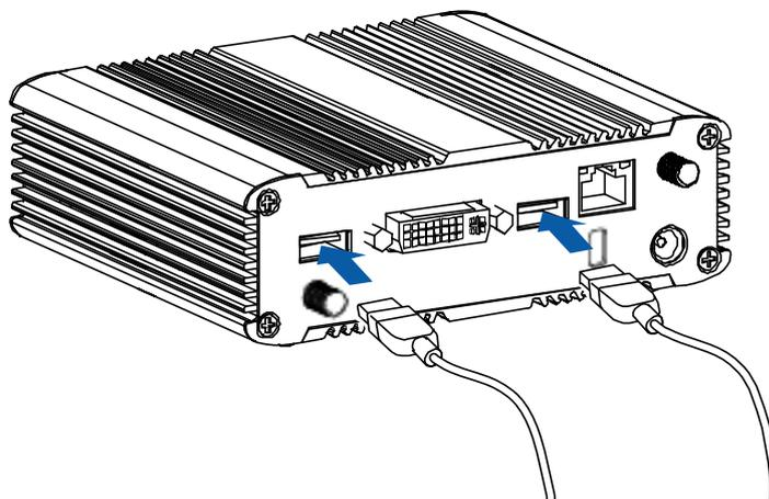
Figure 5 Connecting USB mouse & keyboard
