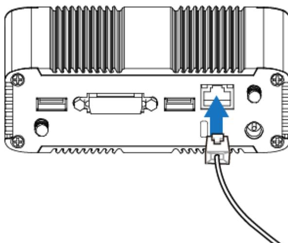
Figure 6 Network cable with RJ45 connector
