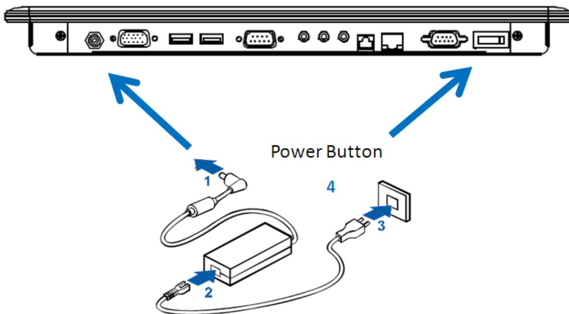
Figure 7 Turning on the system
