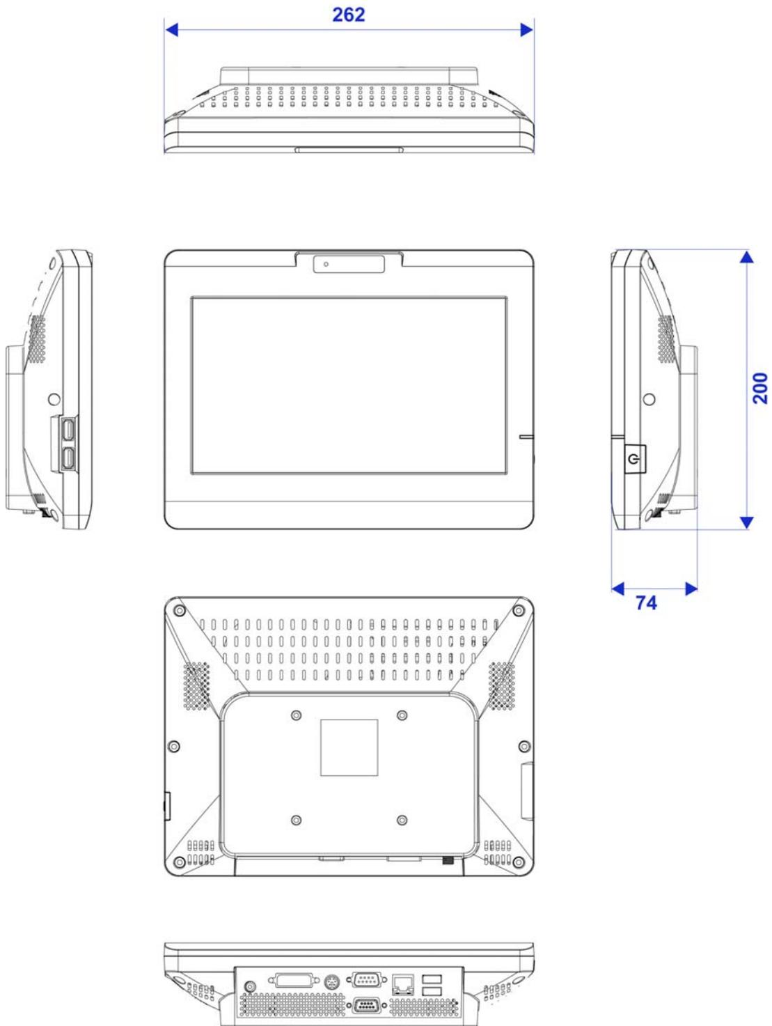
Figure 3 Mechanical Dimensions
