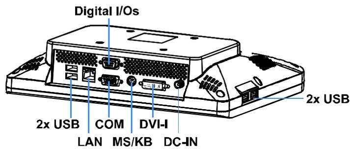
Figure 2 Mechanical Layout - I/O Panel
