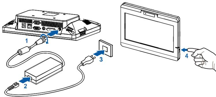
Figure 4 Turning on the system
