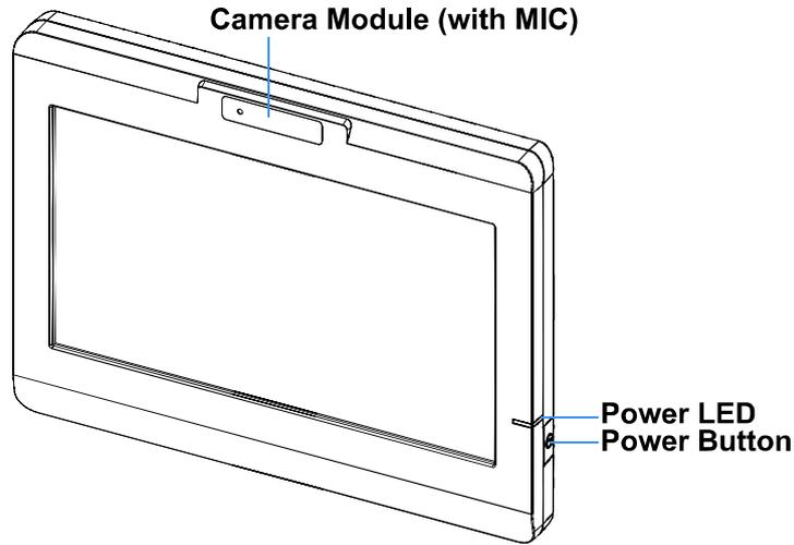
Figure 1 Mechanical Layout - Front and Side
