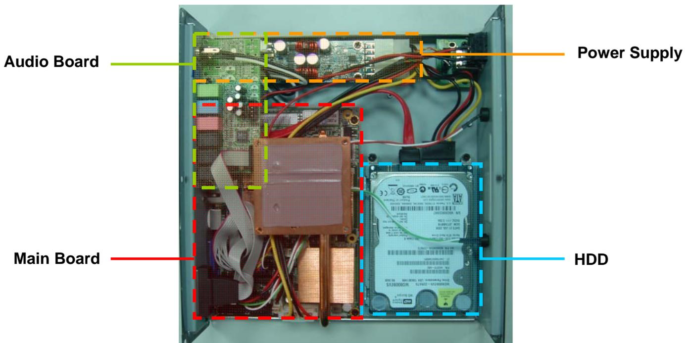
Figure 2 Mechanical Layout - Internal Components
