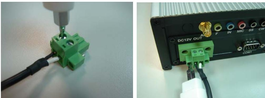
*Figure 10 Tighten the terminal block compression clamps, insert into the DC inlet and secure*
