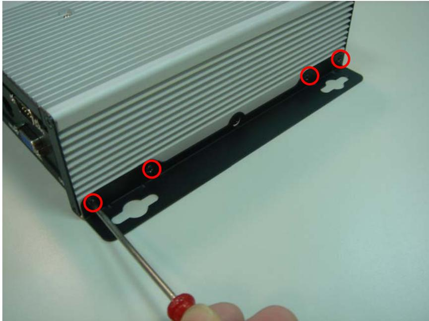
Figure 7 Secure the L-brackets for wall mounting
