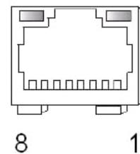
Table 7 Gigabit Ethernet Connector (LAN1: RJ-45)
