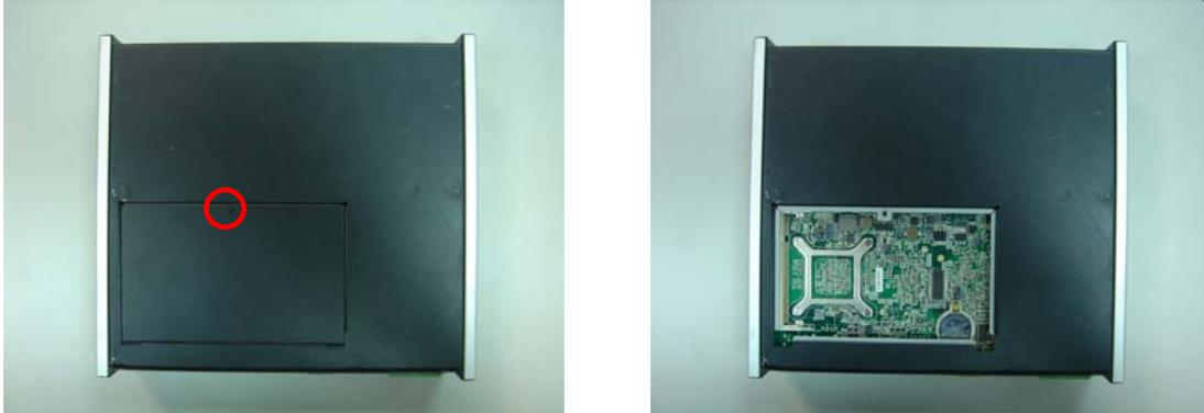
Figure 3 Remove chassis bottom cover
