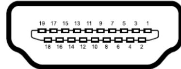
Table 5 HDMI Panel Connector (HDMI1: Type A Connector - 19-pin)
