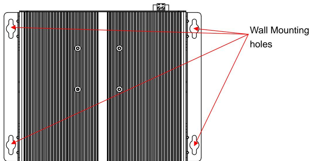
Figure 8 Wall mount holes spacing
