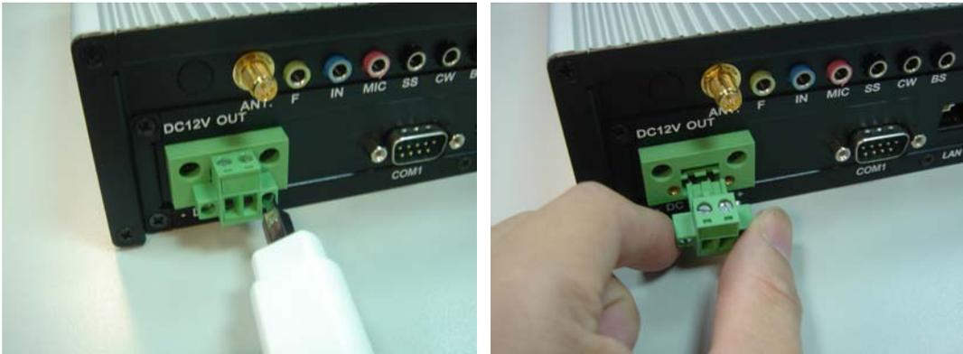
*Figure 9 Loosen screws securing DC terminal block and remove from chassis*
